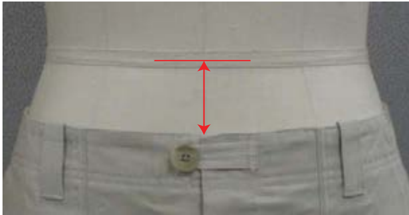
This measurement is for fit reference on the dressform. Measure from Center of waist tape on dressform to top edge of garment waist at Center Front.
