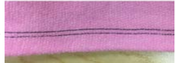
Internal View: 2N to inside, no loops
