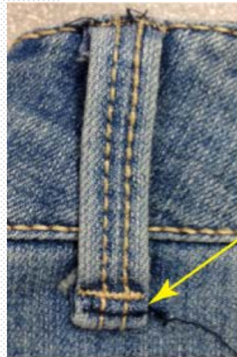
Pre-setting beltloops before bartack. Looks poorly executed and doesn't achieve consistent beltloop length
