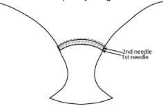
• **Flatlocked crotch seam** should be tacked the full width of the flatlock seam. The thread tail should be pulled back and caught under the bartack. The seam should be tacked with a 28 stitch bartack.
