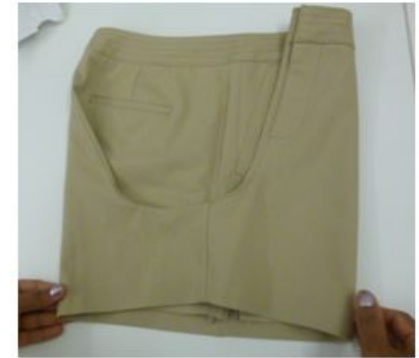
Saddle is unbalanced and off from the center
