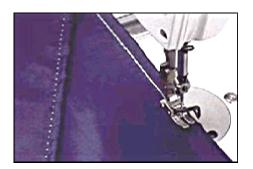
**DESCRIPTION:** Fagoting units the finished edges of two pieces of fabric with a space between the edges using a decorative chainstitch. In this case, a Duplex (double needle) ISO 411 stitch is used.
